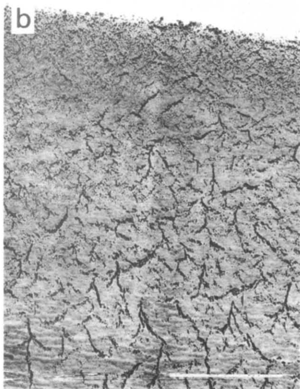
Figure 4 Micrographs of transverse sections through stained Kevlar 29 (a) and Kevlar 49 (b), respectively. Scale markers 1.0 \mu\text{m} and 0.5 \mu\text{m}
